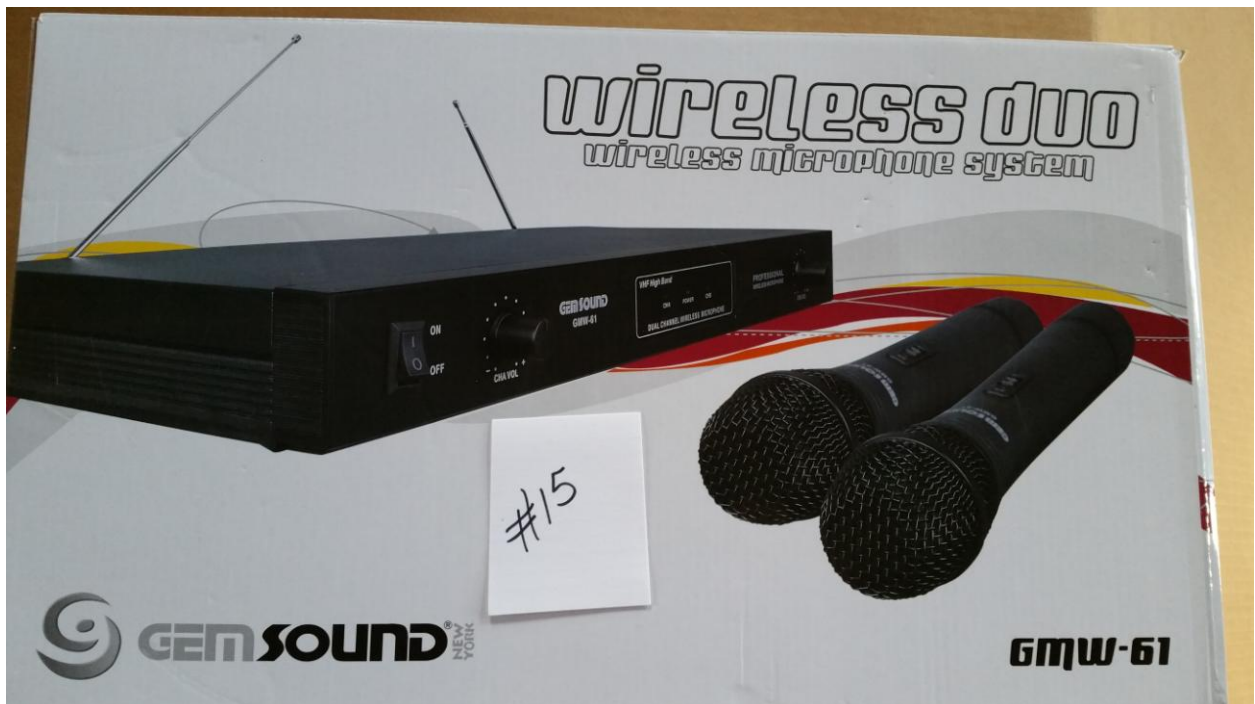
#15 – GemSound wireless mic system, GMW-61: 2 HH wireless mics, receiver, 'out' cable + extra cable in box that belongs to something else. VHS system; takes 9V battery
